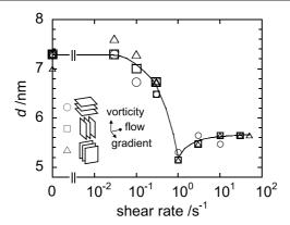
Figure 1. Shear rate dependence of the repeat distance for the vorticity (O), transverse  $(\Box)$ , and parallel  $(\triangle)$  orientations previously reported [20]. The different symbol sizes correspond to different runs.
