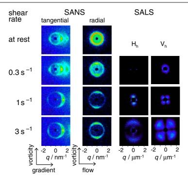
**Figure 2.** Evolutions of 2D patterns of SANS [20] and polarized  $(H_h)$  and depolarized  $(V_h)$  SALS with increasing shear rate, from 0 to 3 s<sup>-1</sup>. No significant scattering pattern is observed at rest for SALS
