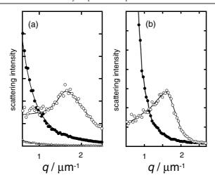
Figure 3. 1D polarized  $(H_h)$  and depolarized  $(V_h)$  SALS patterns for the shear rates of  $0.3 \,\mathrm{s}^{-1}$   $(\triangle)$ ,  $1 \,\mathrm{s}^{-1}$   $(\bullet)$ , and  $3 \,\mathrm{s}^{-1}$  (O) obtained by integrating the 2D scattering intensity over a segment of width  $\Delta \phi = \pm 10^{\circ}$  where  $\phi$  is the azimuthal angle.
